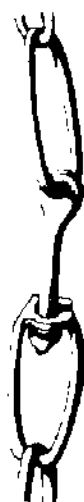
FIGURE 4. Piece of chain, showing the swivel: Hereford. [From John Clark, The Care of Books , Cambridge Univ. Press, 1901.]
