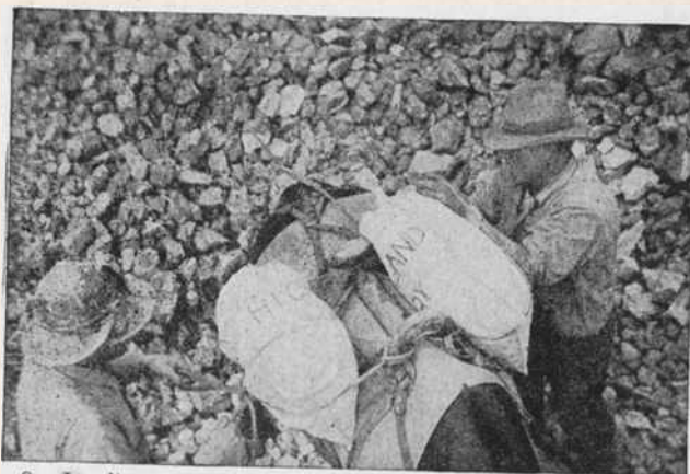
FIG. 8.—Loading ore. Steel hangers may be used in place of ropes. (Courtesy of George O. Argall, Jr.)
