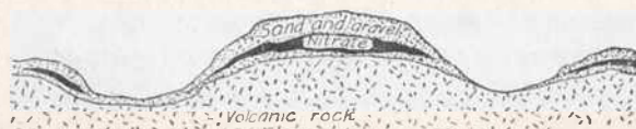
FIG. 105.—Section of a Chilean nitrate deposit. The overburden may be from a few inches to several feet deep, after which may be several feet of low-grade caliche (nitrate), then up to 6 feet of the workable caliche, and underlying the whole is volcanic rock.
