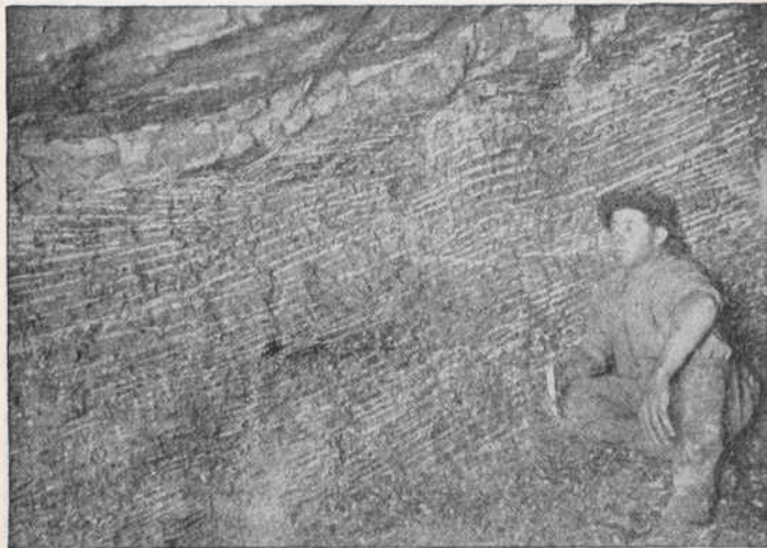
FIG. 97.—Characteristic occurrence of chrysotile asbestos in serpentine. New Amianthus mine, eastern Transvaal, South Africa. (From South African Mining and Engineering Journal .)
