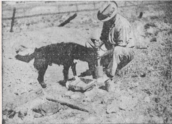
FIG. 21.—A simple and workable sampling outfit—a short mercury flask for mortar, drill-steel for pestle, sieve tacked to a frame, and pan.
