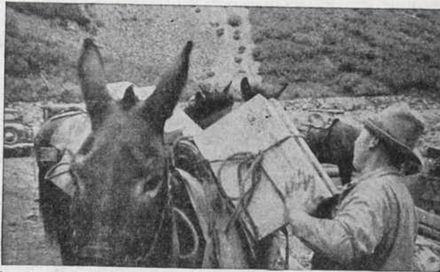
FIG. 6.—Loading dynamite. In loading two boxes or other articles it is important to bring the rope under both to prevent them from dropping out. (Courtesy of George O. Argall, Jr.)
