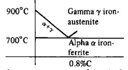
If the steel is held for the necessary amount of time in the austenitic state, then all the iron carbide present in the steel will be dissolved and held in solution in the austenite.
