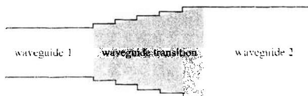
Figure 32. Waveguide transition obtained by tapering. As one can see, the mode matching approach replaces the continuous tapering by a finite set of abrupt transitions.
