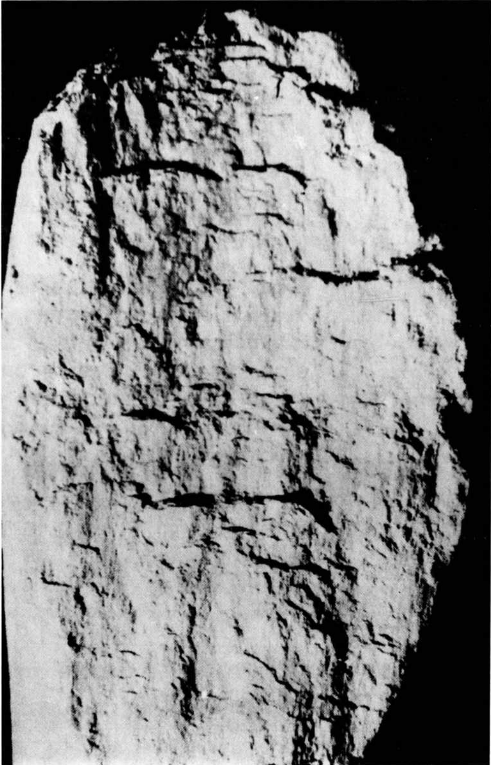
Fig. 11-19. Slickensides and small steps or ridges developed on shear surfaces (after PATERSON, 1958).
