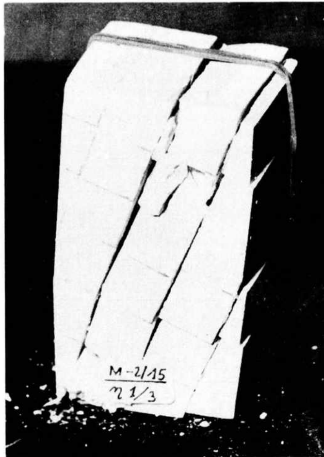
Fig. 10-114. Fracture of a jointed model with joint inclinations \kappa_1 = 15^\circ , \kappa_2 = 75^\circ , \chi = 1/3 , showing failure along \kappa_1 joint (after LAMA, 1975 a).
