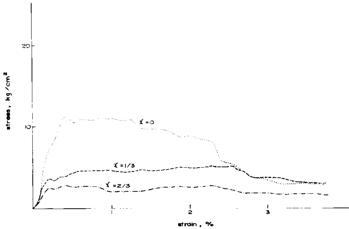
Fig. 10-112. Stress-strain curves for joint inclination angle \phi = 45^\circ with different values of \gamma (after LAMA, 1975a).
