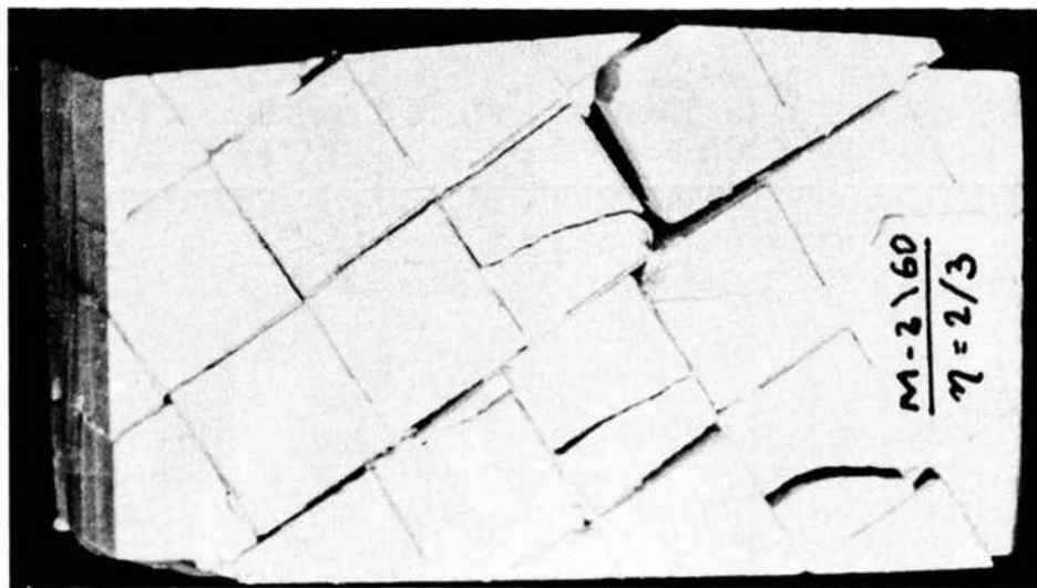
Fig. 10-115. Fracture of a jointed model with joint inclinations \kappa_1 = 60^\circ , \kappa_2 = 30^\circ , \lambda = 2/3 , with failure along \kappa_2 joint and with development of secondary fractures originating from joint interfaces (after LAMA, 1975a).
