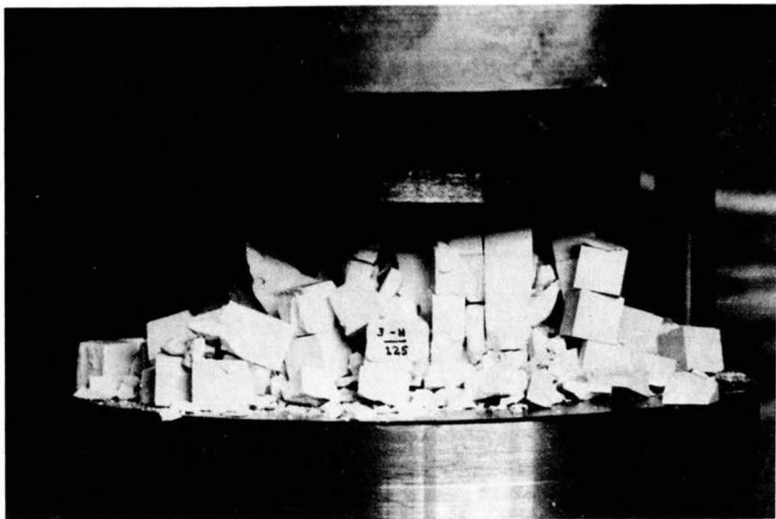
Fig. 10-106. Jointed model ( n = 125 ) at 30% of strain showing presence of some blocks still intact (unfractured) (after LAMA, 1974a).
