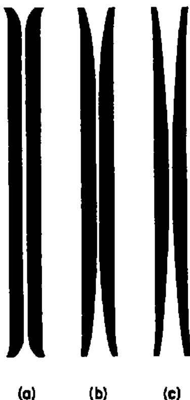
FIG. 2.3. Shapes of capillaries in viscometers after Caw and Wylie.
