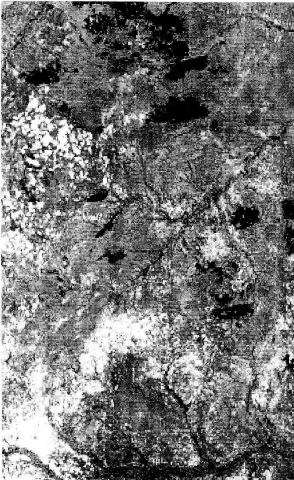
FIGURE 6 TM imagery of Burkina Faso (Kaibo area). Acquisitions: 26 October 1989 (a) and 3 March 1987 (b). (a) white, bare soil and dry grass + weeds; light grey, dry grass, shrubs, and trees; grey, shrubs and trees with dry grass; dark grey, crops and abundant trees + shrubs; black, burned savanna area. (b) white, bare soil and dry grass + weeds; light grey, dry grass, shrubs, and trees; grey, shrubs and trees with dry grass; dark grey, abundant green trees in valley bottoms; black, burned savanna area.
