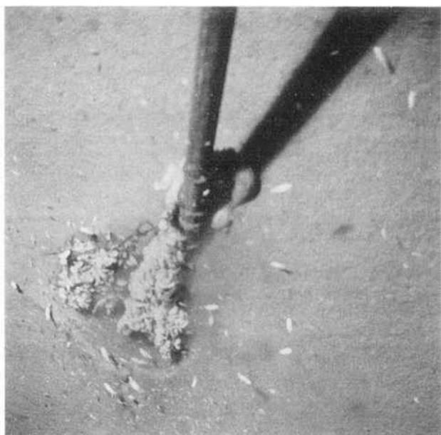
Fig. 4. Photograph of amphipods swarming to food (dead fish) placed on the seafloor at a depth greater than 10,500 m. The dead fish were tied to one end of an expendable pole and the 35 mm camera in a pressure-resistant housing was mounted at the other end of the pole by means of a time-release mechanism. The pole and other ballast were left on the seafloor when the time-release mechanism was activated to enable the floats to raise the camera to the sea surface. The amphipods are Hirnodellea gigas . Pictures such as this one suggest that the animals inhabit this depth. But this does not prove that the animals reproduce at this depth. These animals were not able to survive decompression to even 34 MPa in the few experiments conducted.
