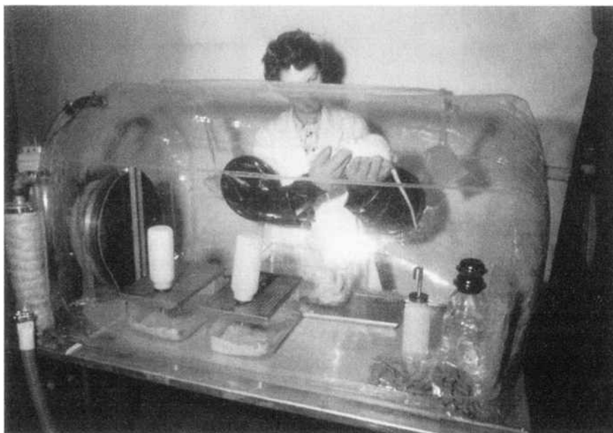
Fig. 3. Plastic isolator with air filter in foreground and outlet trap partially visible behind the filter.
