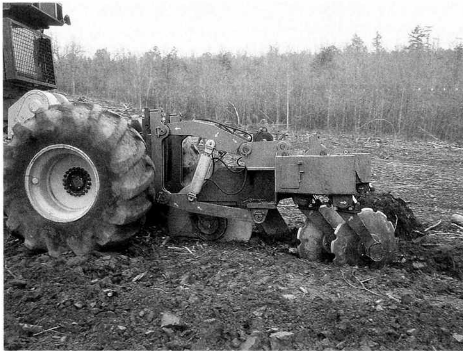
Figure 8 Subsoiling plow used for forest tillage to prepare soil before tree planting. Note backward sweep of subsoiler shank, which is used to allow the implement to pass over tree stumps.
