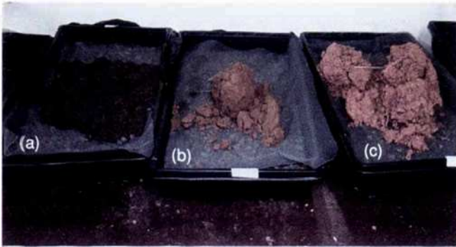
Plate 56 Structure Fragmentation state of large clods after six wetting-drying cycles: (a) clayey vertisols; (b) clayey oxisols; and (c) clayey ultisols.
