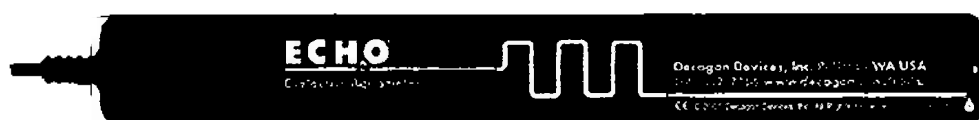
Figure 1 An example of a capacitance soil-water content sensor. The circuitry to measure the capacitance is in the overmolded head of the probe. The capacitance sensor is in the blade and consists of parallel conductors sandwiched between insulating layers.
