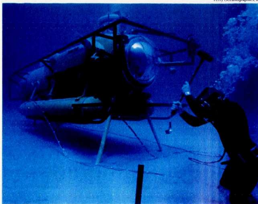
An underwater diver drives a device into the ocean floor to obtain samples of the ocean bottom for research. The diver descended in a vehicle called a submersible . Two cables link the diver to the submersible. One supplies breathing gas, and the other enables the diver to communicate with people in the vehicle.
